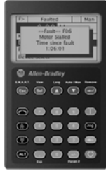
LCD Display, Full Numeric Keypad 20-HIM-A3
