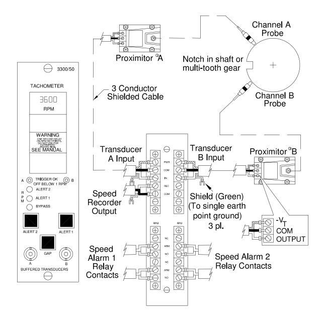
Figure 1: Field wiring diagram for 3300/50 Dual Setpoint Tachometer
