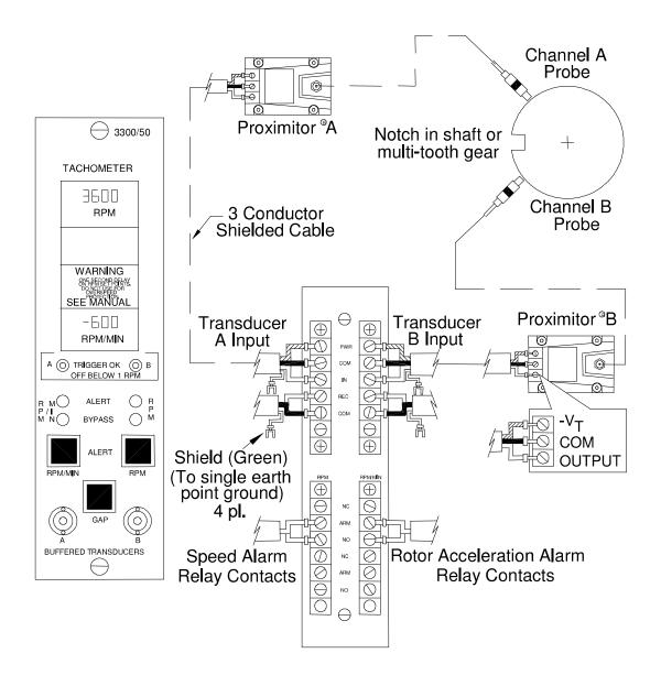
Figure 3: Field wiring diagram for the 3300/50 Rotor Acceleration Tachometer
