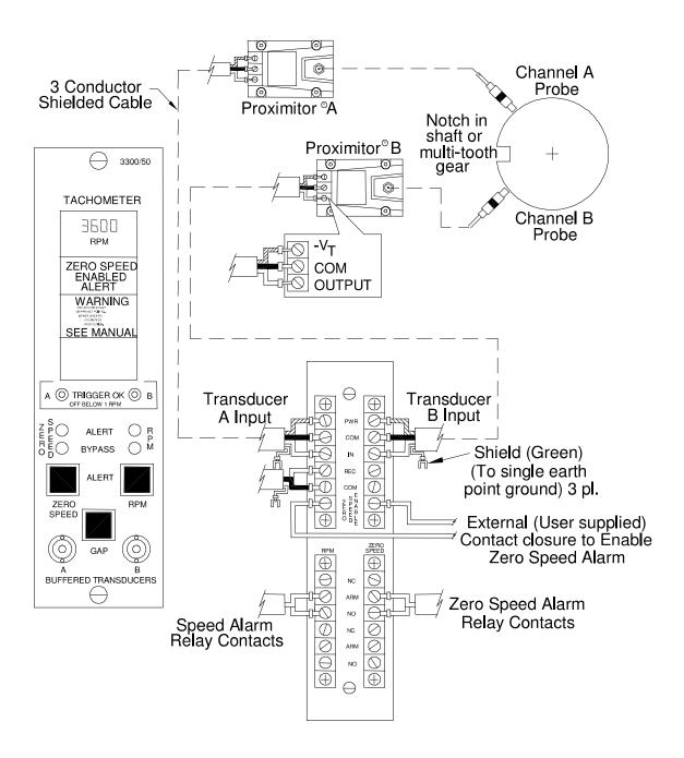
Figure 2: Field wiring diagram for the 3300/50 Zero Speed Tachometer
