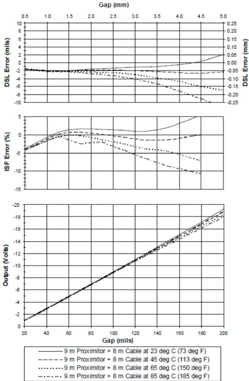
**Figure 8: Typical 3300 XL 11 mm 9 m Proximito with 8 m of Extension Cable @ High Temperature**
