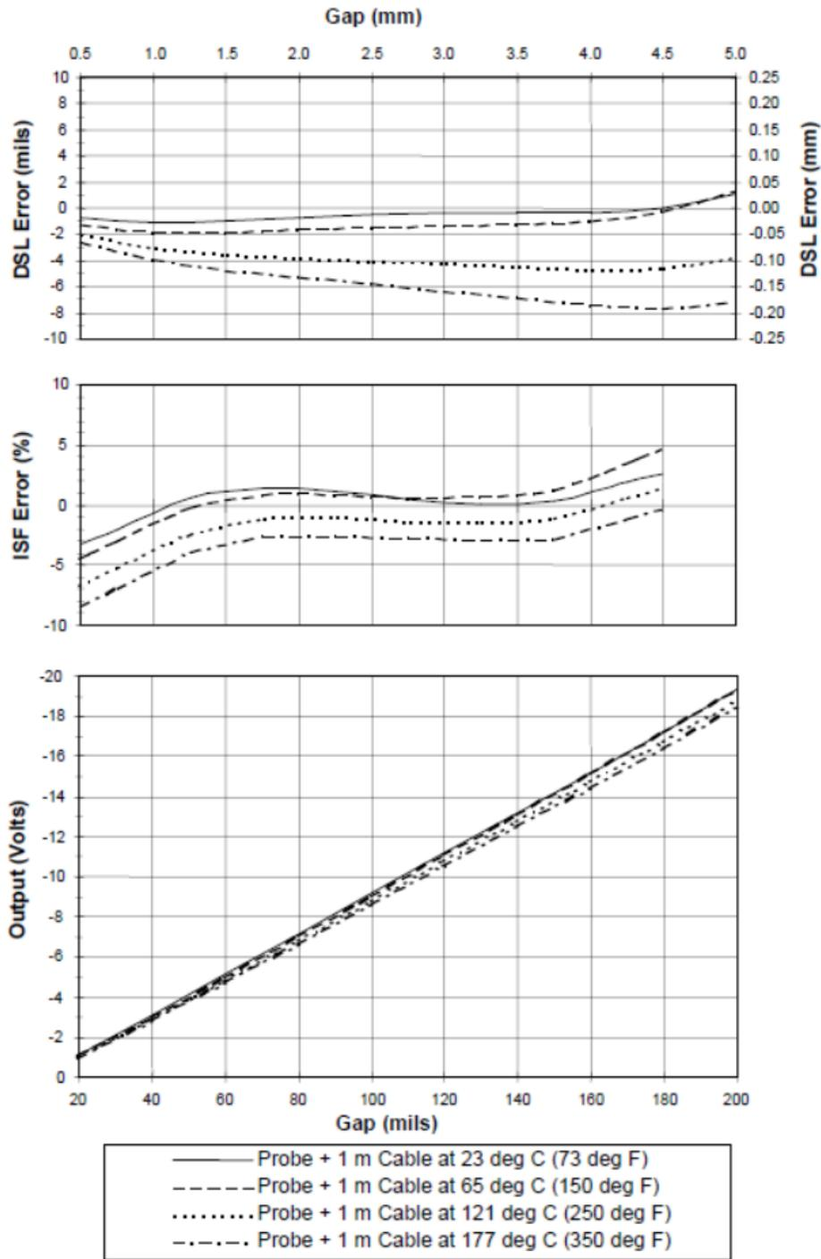
**Figure 4: Typical 3300 XL 11 mm Probe + 1m Cable @ High Temperature**
