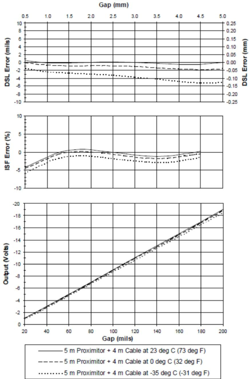
**Figure 5: Typical 3300 XL 11 mm 5 m Proximator Sensor with 4 m of Extension Cable @ Cold Temperature**
