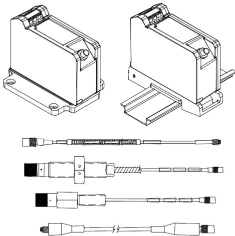
The 3300 XL 11 mm Proximity Transducer System has a 3.94 V/mm (100 mV/mil) output for non-contacting vibration and displacement measurements on fluid film bearing machines. The large 11 mm tip enables this transducer system to have a longer linear range compared to our standard 3300 XL 8 mm Transducer System. It is primarily used in the following applications where the longer linear range is necessary:
