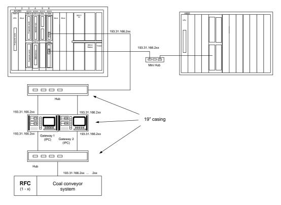
The hardware configuration of the TCP/IP coupling is shown below:
