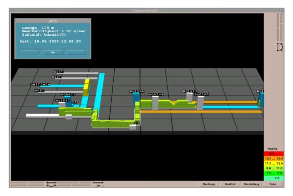
The transport model permits continuous tracking in space and time of the coal flow and its quality data on the conveyor lines from the mining machines or the bunker.
