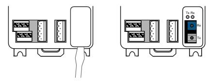
Figure 3 (Left) Removing the protective lid of the TB81x bay. (Right) TB81x Optical ModuleBus Port inserted.
