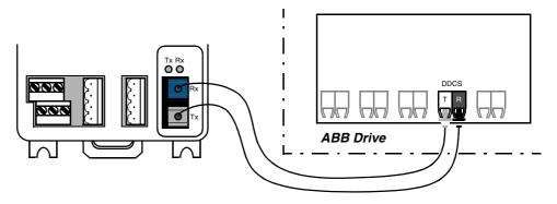
Figure 4 Fibre optic link connecting the FCI to the drive.
