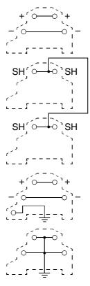
Figure 2 TC505 internal connections.
