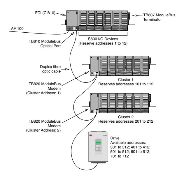
Figure 5 An example of device addressing on an Optical ModuleBus link.
