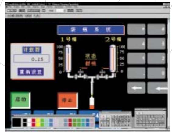
PanelBuilder32 development software can be used to configure application screens with text in over 46 languages
