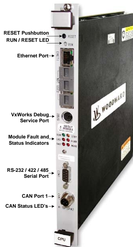
Figure 6-8—CPU5200L Module
