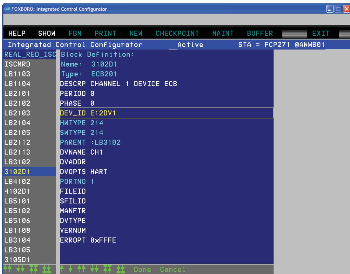
Figure C-6. Creating an Device ECB201 for a LB 3102 Module (Example)
