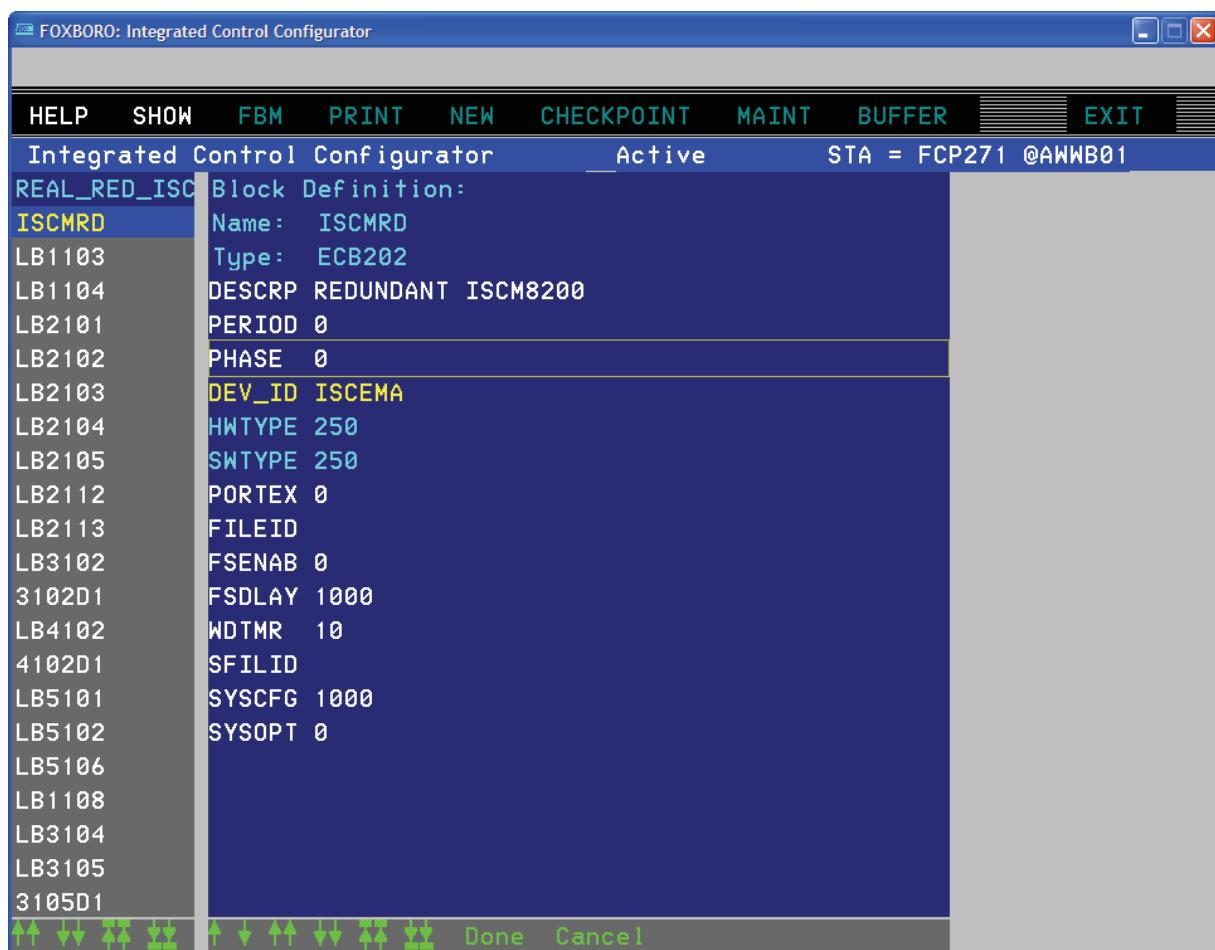
Figure C-2. Creating an ECB202 for a Redundant ISCM in ICC (Example)
