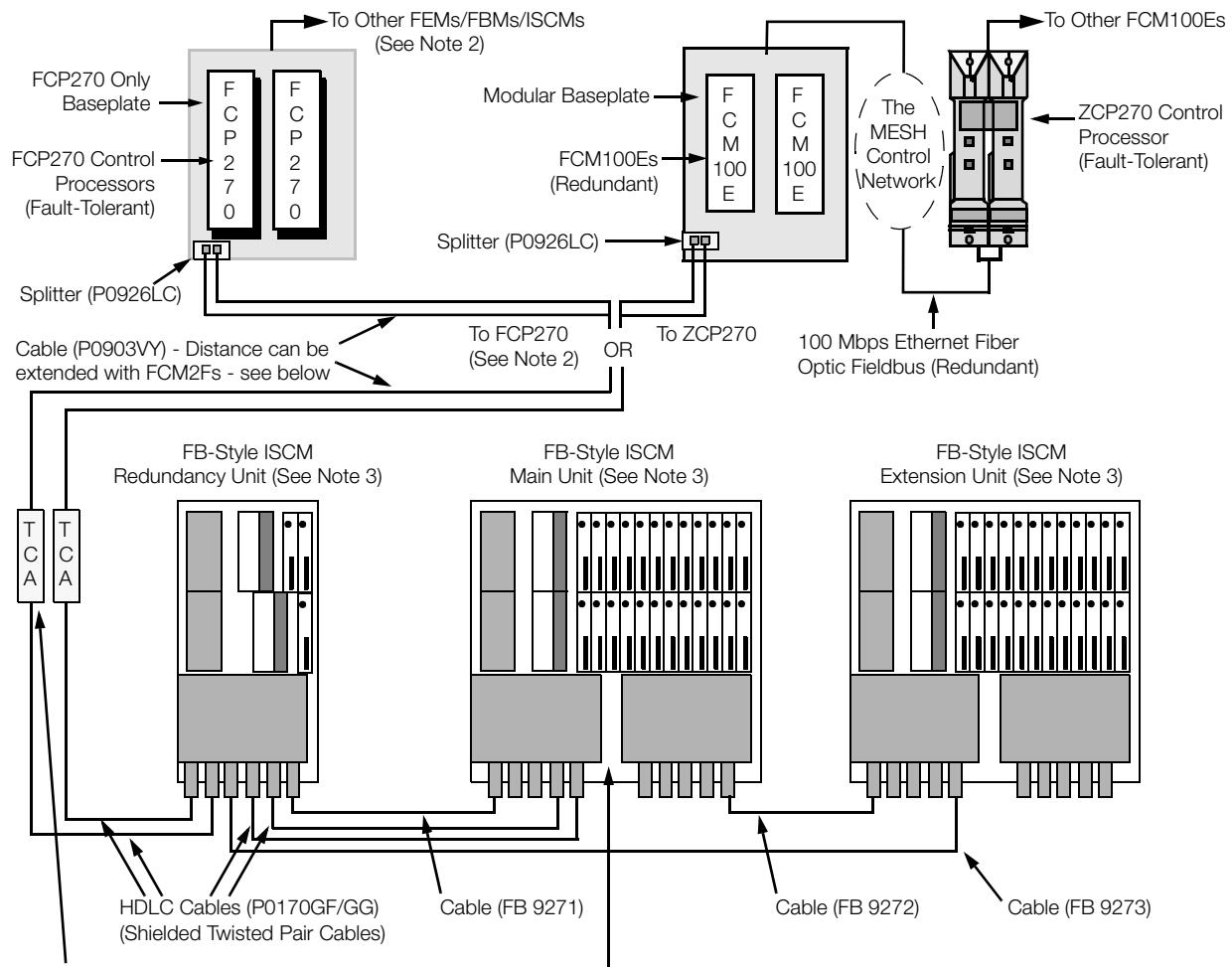
110 Ohm Terminations at Each End of the HDLC Cables (152 m (500 ft) Max.) - TCA is on the P0903VY cable
