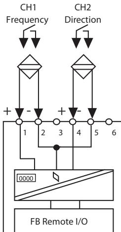
Figure B-17. FB 1303 F and FB 1303 F2 Input Connections
