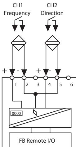
Figure B-14. FB 1203 FL Input I/O Connections
