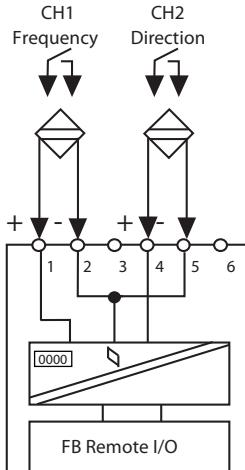
Figure B-16. FB 1204 FL Input Connections
