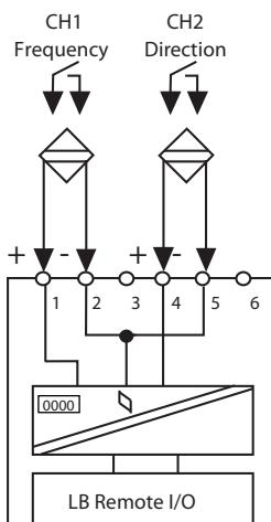
**Figure B-3. LB 1103 F Input Connections**
