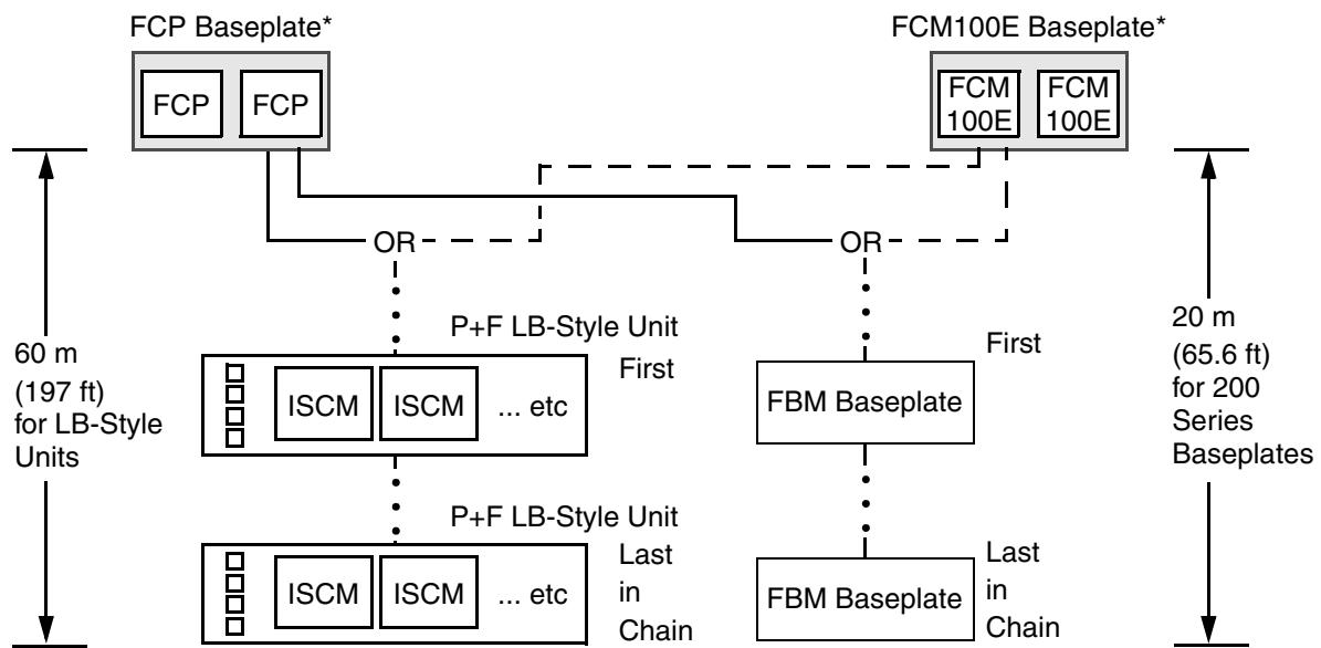
**Figure 1-8. Fieldbus Cable Length Restrictions for FCP270, FCM100E and LB-Style Intrinsically Safe Units**
