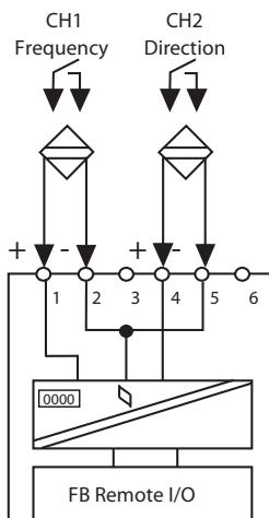
**Figure B-19. FB 1304 F and FB 1304 F2 Input Connections**
