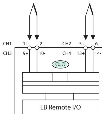
**Figure B-12. LB 5105 F Input I/O Connections**
