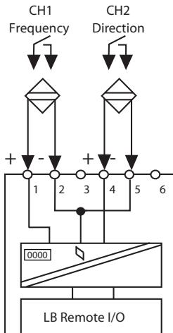
Figure B-6. LB 1104 FL Input Connections
