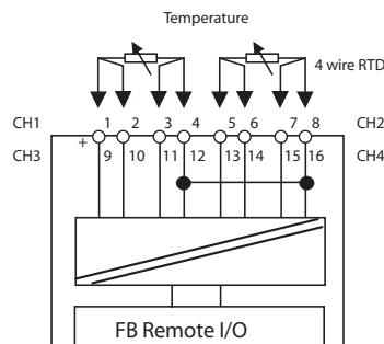
**Figure B-25. FB 5204 F4 Input Connections**
