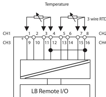
**Figure B-10. LB 5104 F3 Input Connections**
