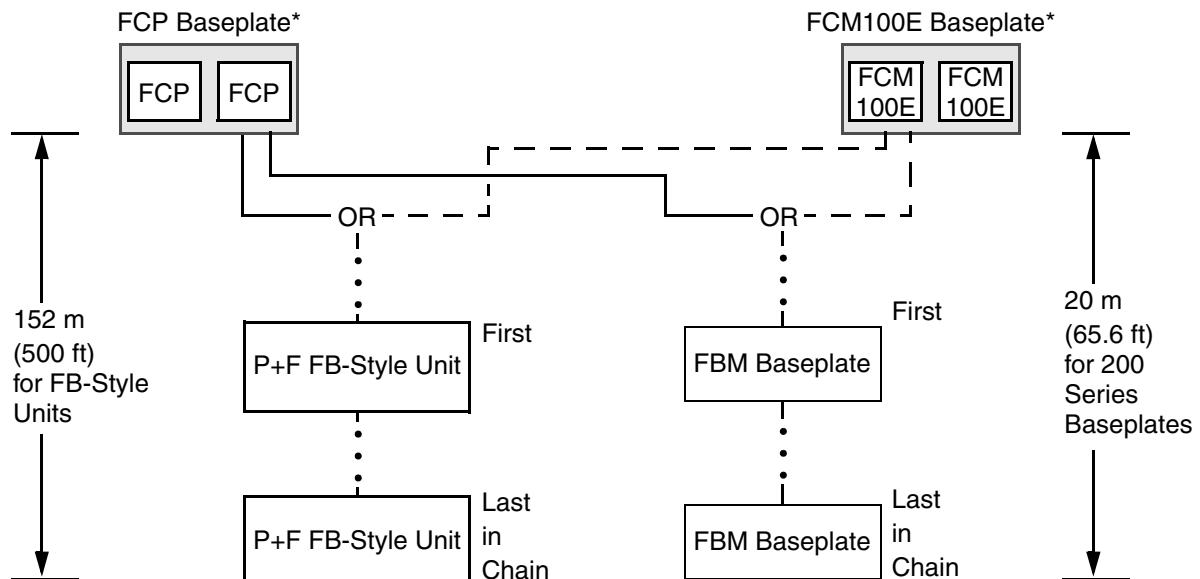
**Figure 1-9. Fieldbus Cable Length Restrictions for FCP270, FCM100E and FB-Style Intrinsically Safe Units**
