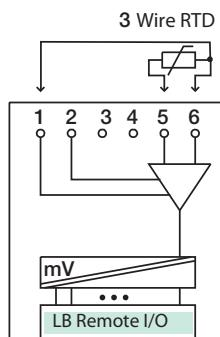
Figure B-7. LB 5101 F3 Input I/O Connections
