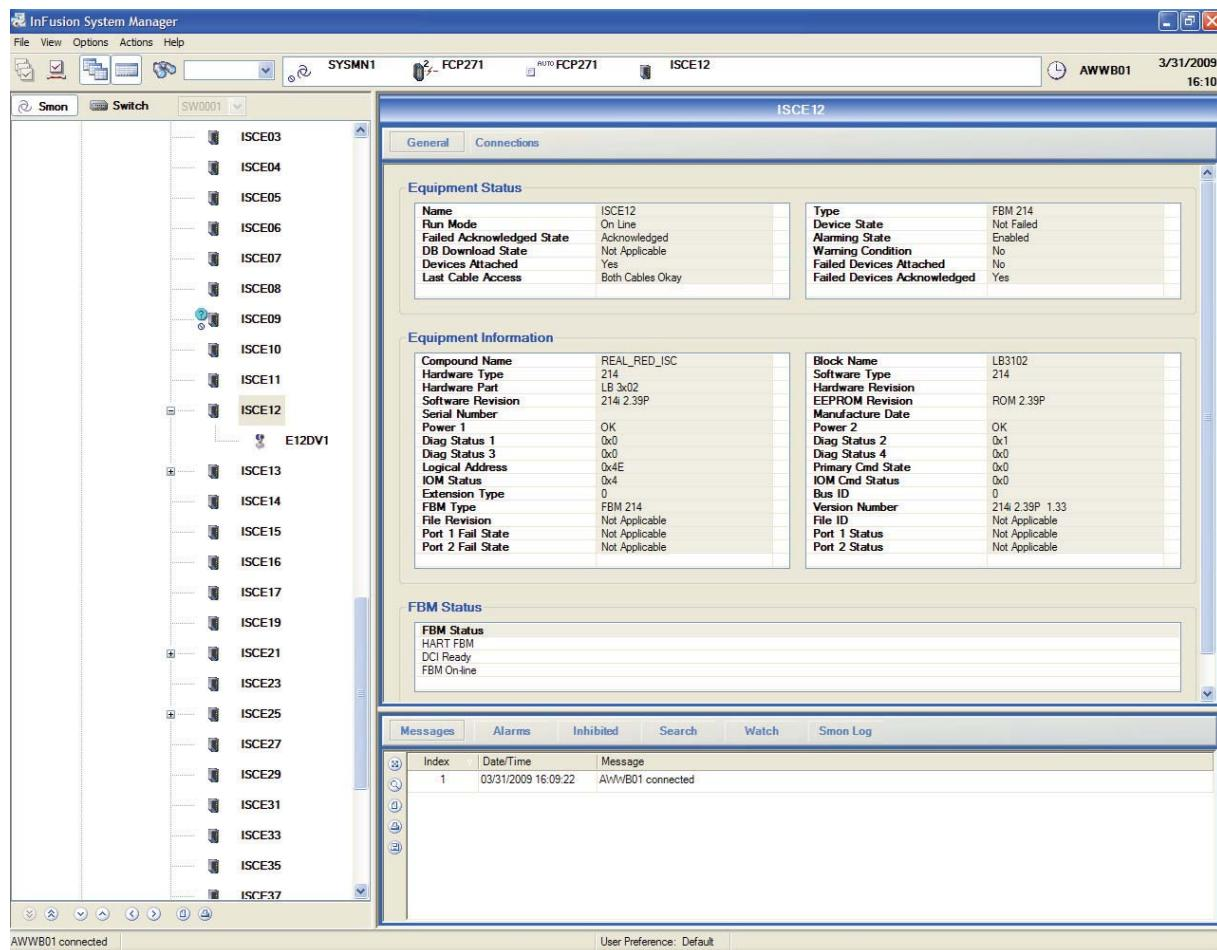
**Figure 5-2. System Manager Display for P+F I/O Modules - Typical**
