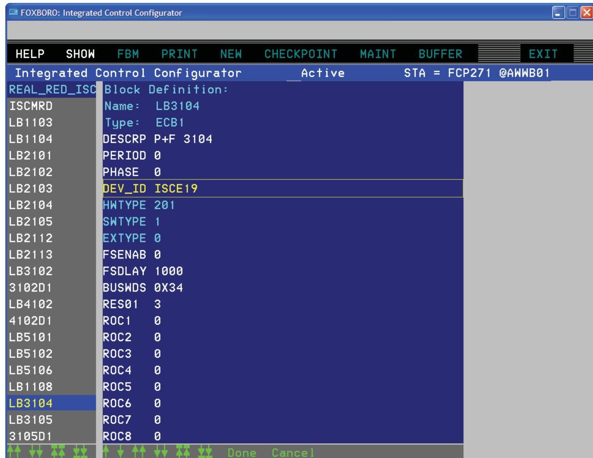
Figure C-3. Creating an ECB1 for a LB 3104 Module (Example)
