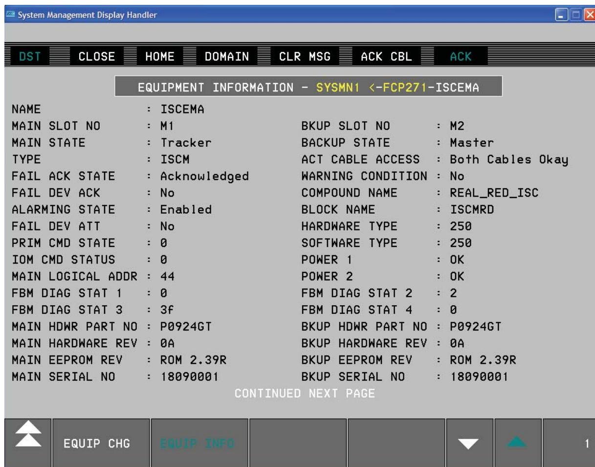
Figure 5-5. Equipment Information Display for ISCM – Page 1 – Typical
