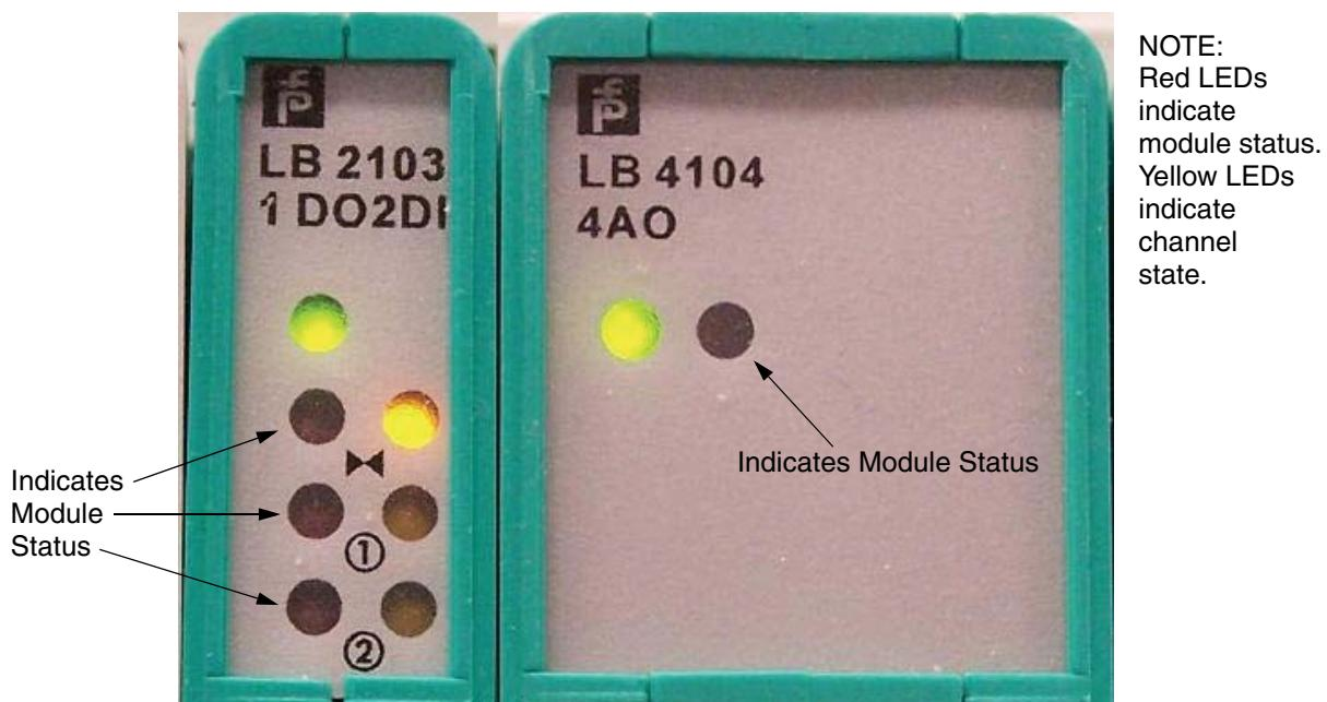
**Figure 6-2. P+F I/O Module LED Indicators**
