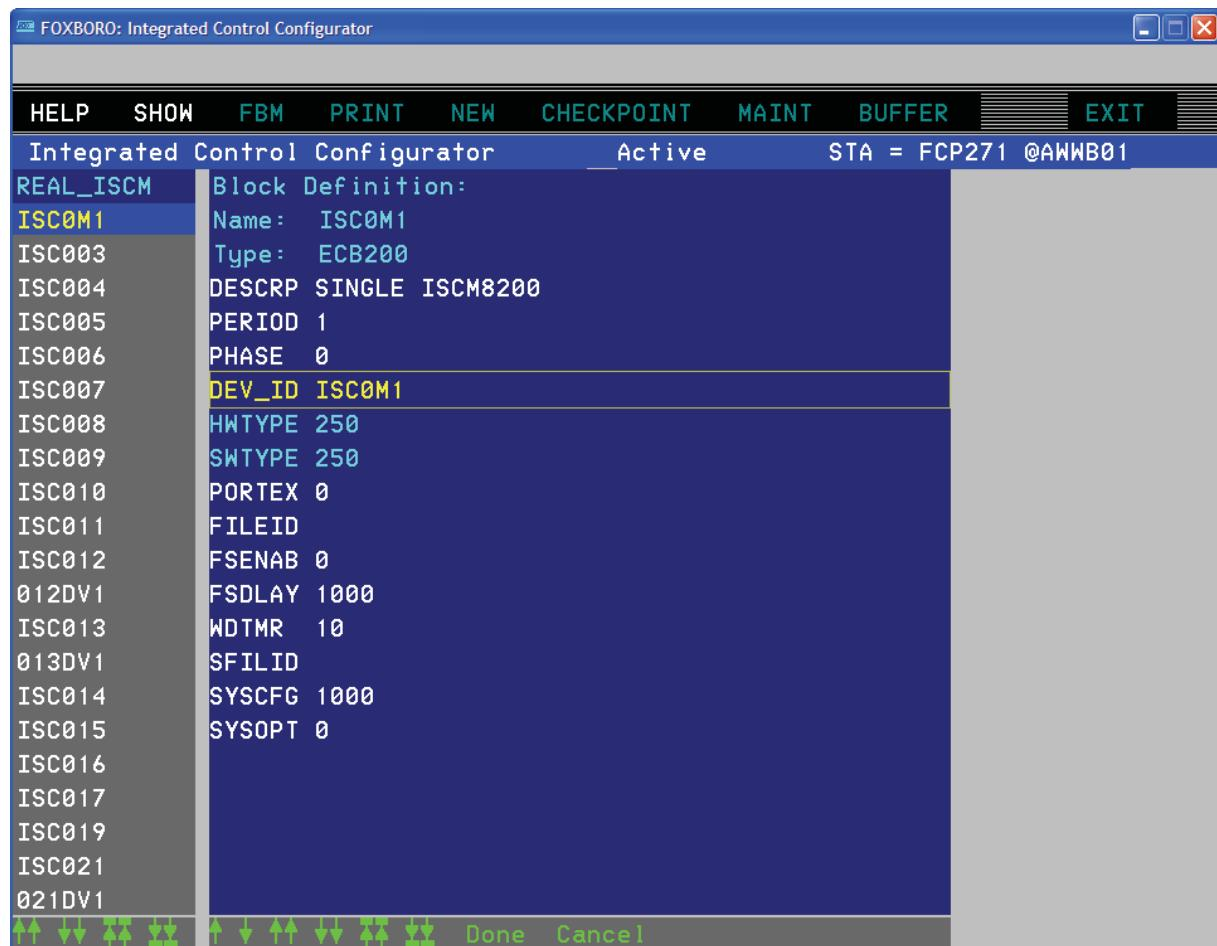
Figure C-1. Creating an ECB200 for a Single ISCM in ICC (Example)
