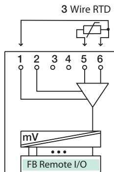
Figure B-21. FB 5201 F3 Input Connections
