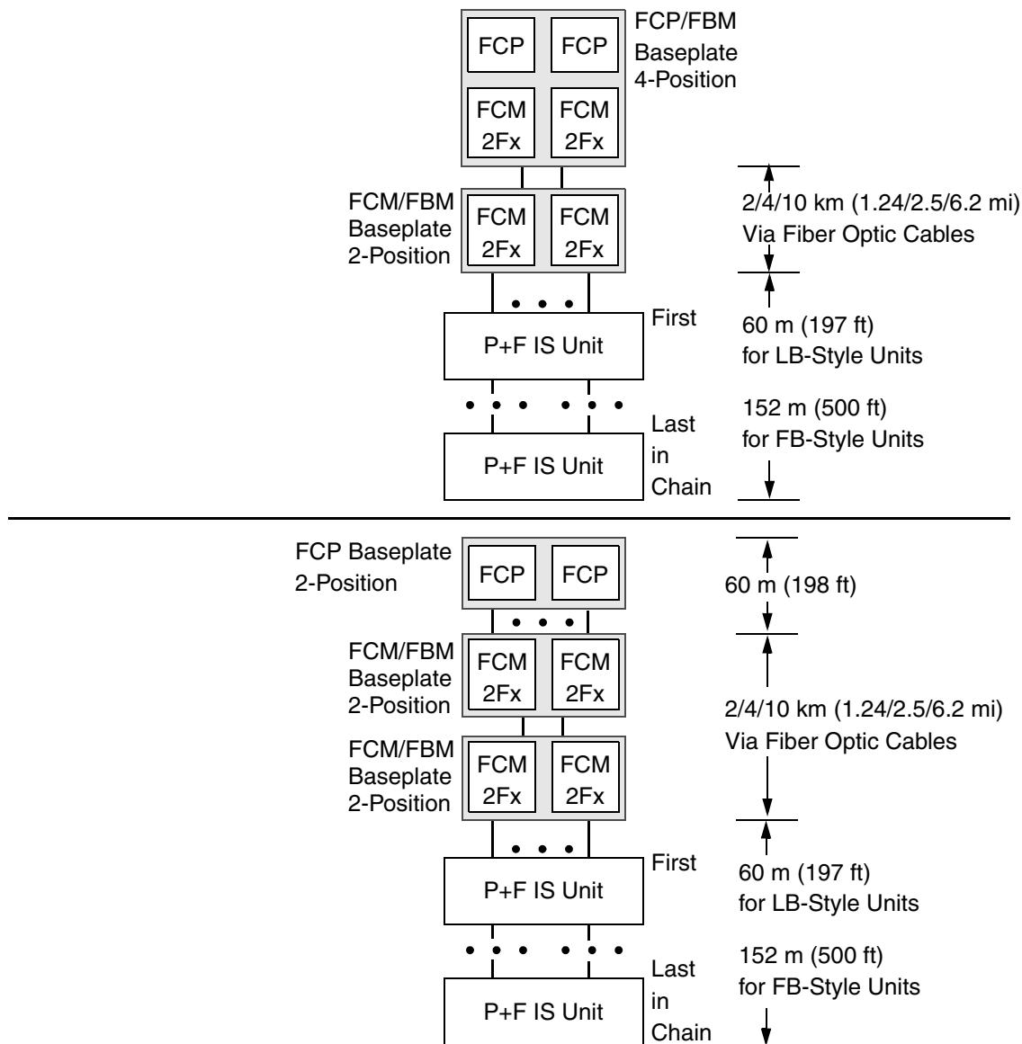
**Figure 1-7. LB-Style and FB-Style ISCM to FCP270 I/O Communications via FCM2Fs (Simplified)**
