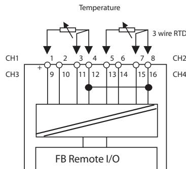
**Figure B-24. FB 5204 F3 Input Connections**
