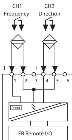
**Figure B-13. FB 1203 F Input Connections**
