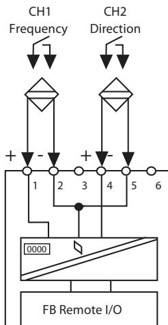
**Figure B-18. FB 1303 FL and FB 1303 FL2 Input Connections**
