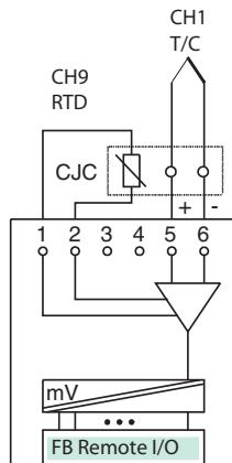
Figure B-23. FB 5202 F Input Connections
