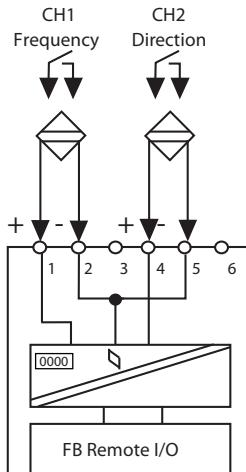
Figure B-20. FB 1304 FL and FB 1304 FL2 Input Connections
