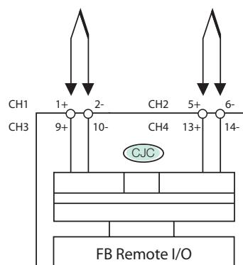
**Figure B-26. FB 5205 F Input Connections**
