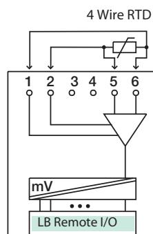
**Figure B-8. LB 5101 F4 Input Connections**
