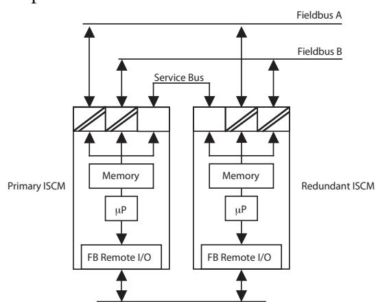
**Figure B-2. ISCM for Zone 1 (FB-Style) Applications (P0924GU) Input Connections**
