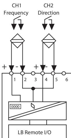
Figure B-4. LB 1103 FL Input Connections
