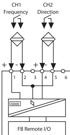
Figure B-15. FB 1204 F Input I/O Connections
