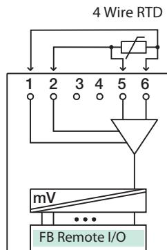
Figure B-22. FB 5201 F4 Input Connections
