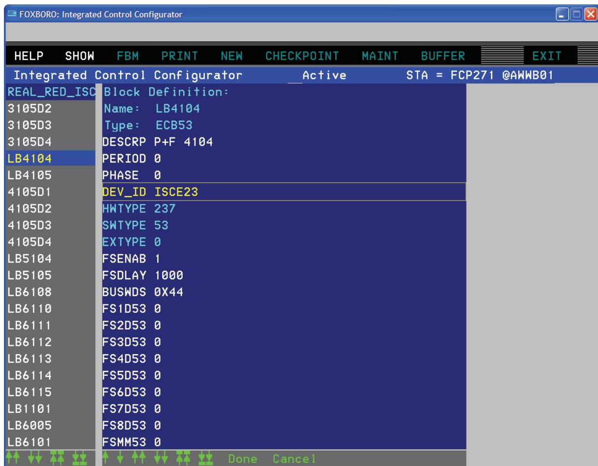
Figure C-4. Creating an EC53 for a LB 4104 Module (Example)
