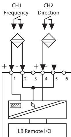
Figure B-5. LB 1104 F Input I/O Connections
