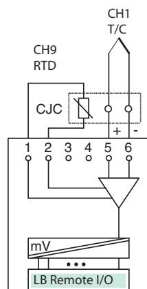
**Figure B-9. LB 5102 F Input I/O Connections**
