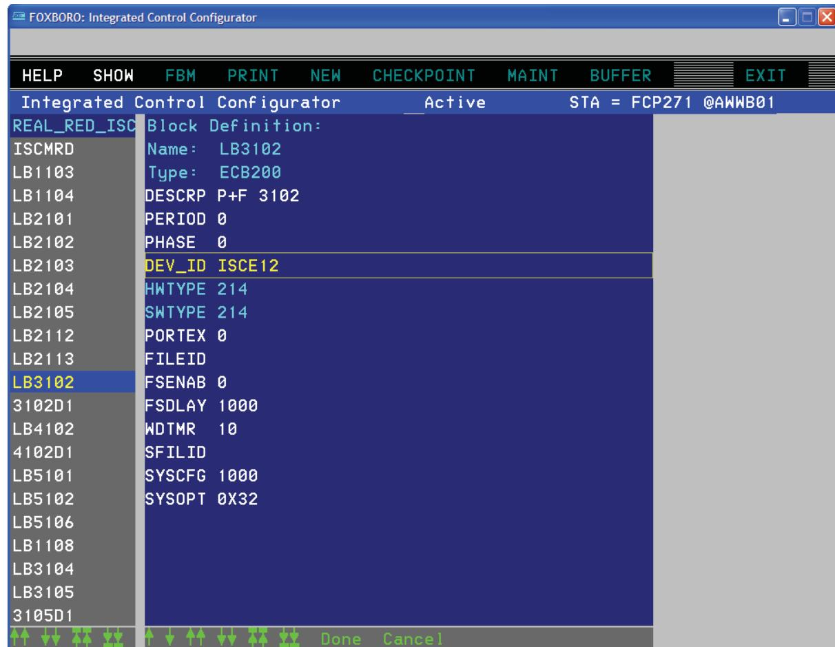
Figure C-5. Creating an ECB200 for a LB 3102 Module (Example)
