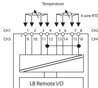
**Figure B-11. LB 5104 F4 Input Connections**
