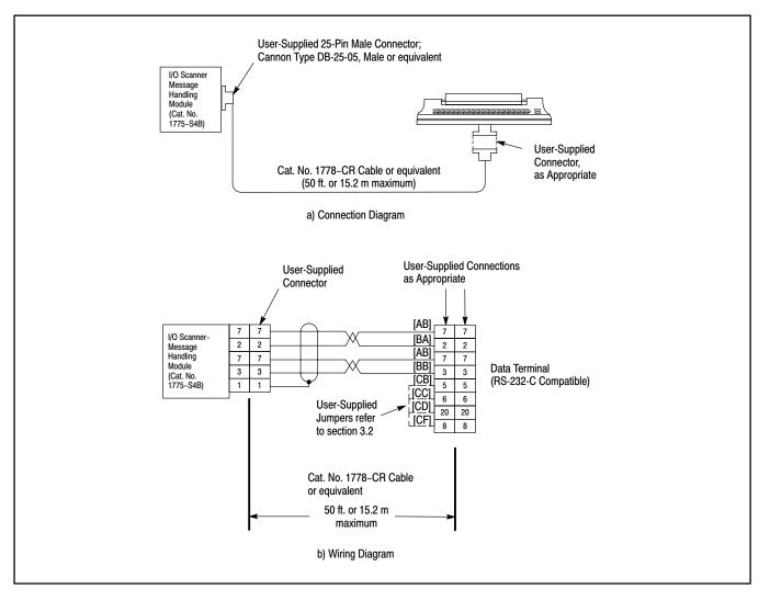
Some RS-232-C devices may require a high signal for a clear to send (CB) signal at pin 5, a data set ready (CC) signal at pin 6, or a data carrier detect (CF) signal at pin 8 for proper operation. Depending on your connections, note the following:
