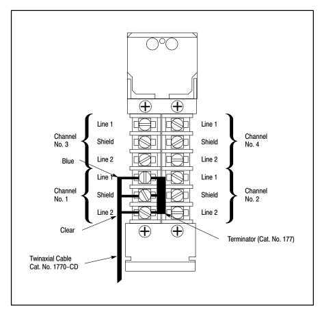
Figure 3.7 shows the terminal identification label which indicates the proper connections for each I/O adapter module to an I/O channel. This label is on the side of the module. The connections are made at screw terminals on a wiring arm in front of each I/O adapter module.
