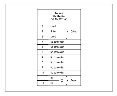
Figure 3.7 I/O Adapter Module (cat. no. 1771-AS) Terminal Identification Label
